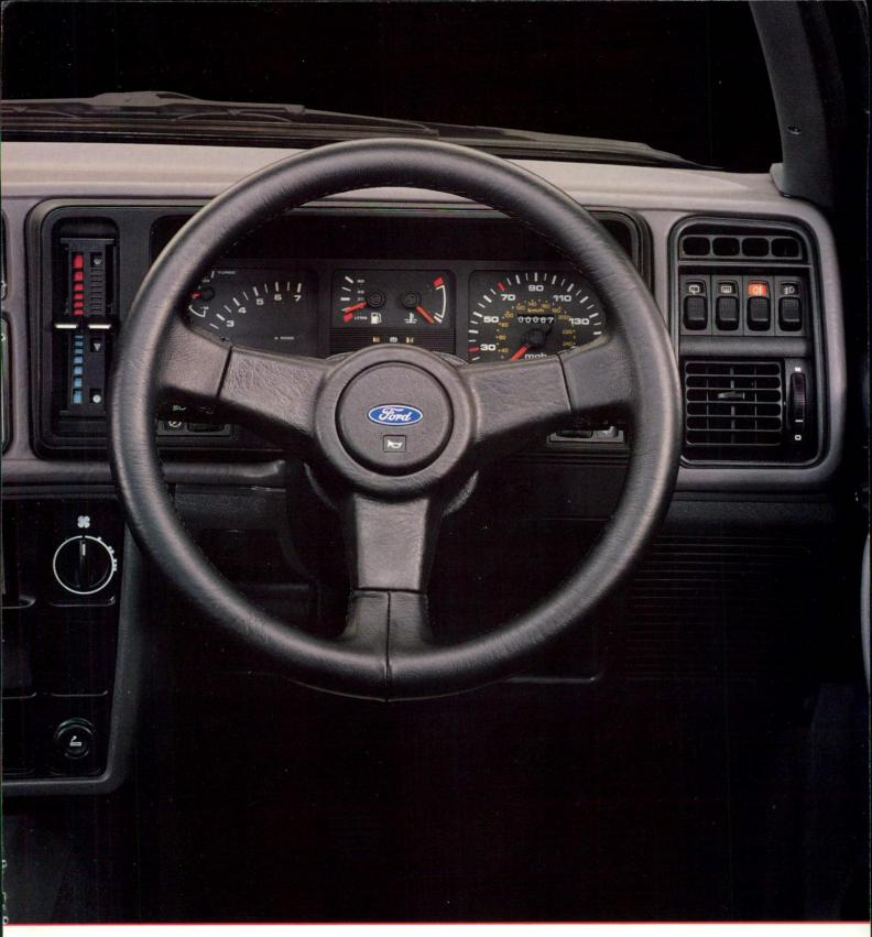
lights are clearly visible through the padded, sportstype steering wheel. Minor controls include a quartet of micro switches to the right of the wheel, and, to the left, smooth-sliding levers for the sophisticated heating and ventilation system. Ford's applied ergonomics make everything easy to see, identify and operate.
