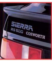
The eye-catching rear wing and tailgate spoiler are features developed to provide increased downforce and stability at racing speeds, and sit well above the discreet Sierra RS 500 Cosworth badging.
