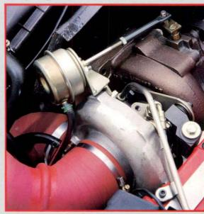
The engines inherent efficiency is boosted by a Garrett AiResearch T31/T04 turbocharger that is mounted onto a special four branch high nickel-alloy manifold. The turbocharger is water cooled to protect the turbo shaft bearings and is set to generate as much low-speed torque as possible.
