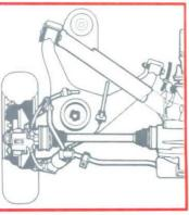
The rear suspension has semi-trailing arms, coil springs, anti-roll bar and gasfilled dampers.
